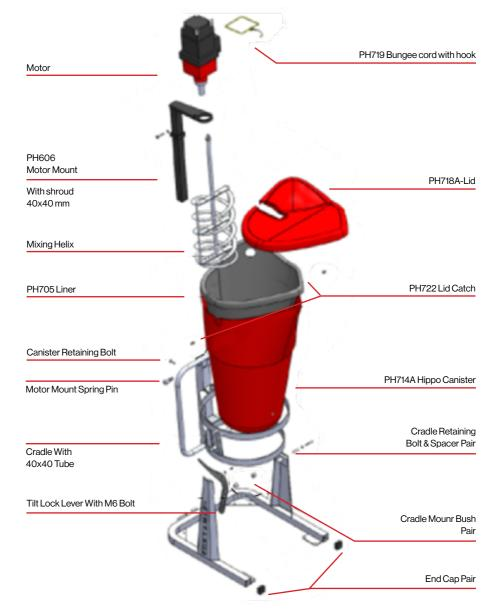
DANGER—SAFETY: Keep hands and other objects well clear of the mixing shaft and canister when mixer is in operation or serious injury could result.
