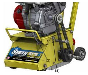
15. Now from the front of the machine observe the motor plate to machine alignment. Tightening the belts with the jackscrew tends to cause the right side of the motor plate to lift higher than the left side. By pushing down on the right front side you can level the plate and then tighten the front right screw to secure in a level position.
