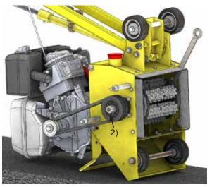
3. Once the hex nuts are off, first support the drum and then remove the shaft by sliding it out towards the sideplate side of the machine. (use precaution as it is HEAVY)
