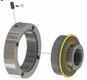
8. Reverse the process and apply thread locking fluid (loctite) to the set screws.
