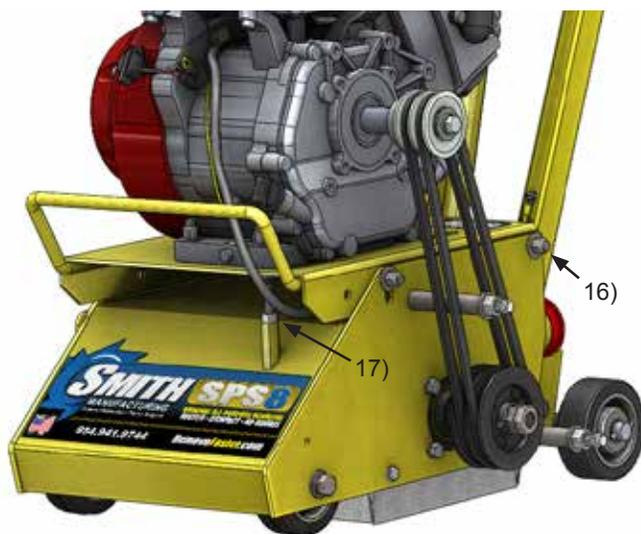
18. Replace the belt cover using the 3/4" box wrench.
