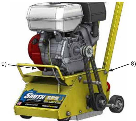
11. Roll the new belt on one groove at a time (two or single multi-groove belt) on both the top and bottom pulleys.
