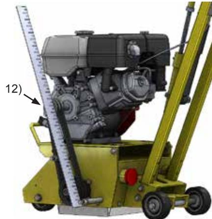
13. After installation, use the 3/8" open-end wrench to screw out the belt tensioning jackscrew under the motor plate to tension the belts to your desired tension. Do not over-tension the belt.
