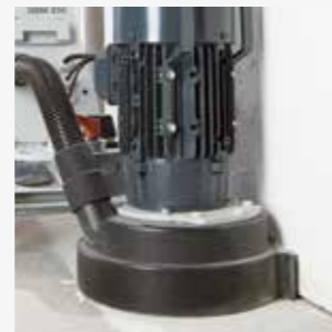
Dust shroud allows you to grind right to the edge while keeping dust under control.
