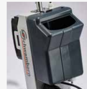
Watertank for wet grinding and polishing.
