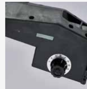
Stepless speed control from 740-1500rpm.
