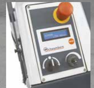
Display with power indication = optimum diamond selection and performance.
