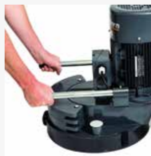
Extendable handles to share weight load when lifting.
