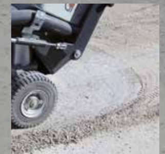
180 degree turning manoeuvres with grinder overlapping to give consistency in your grind or cut.
