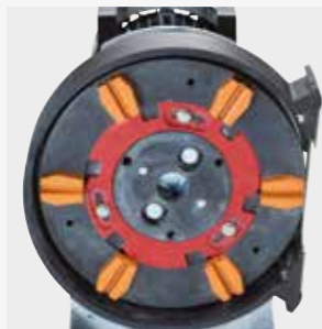
Safety red locking ring holds the diamonds in place when the machine is being transported to or around site.
