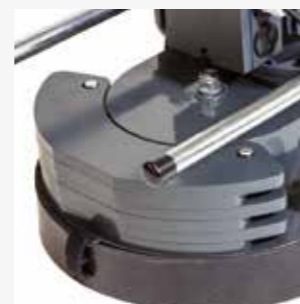
Additional weights for adjustable grinding pressure.
