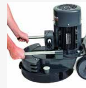
Extendable handles to share weight load when lifting.
