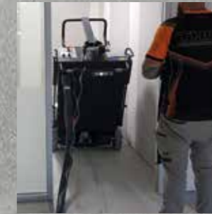
Narrow design to enable tight access through doorways.
