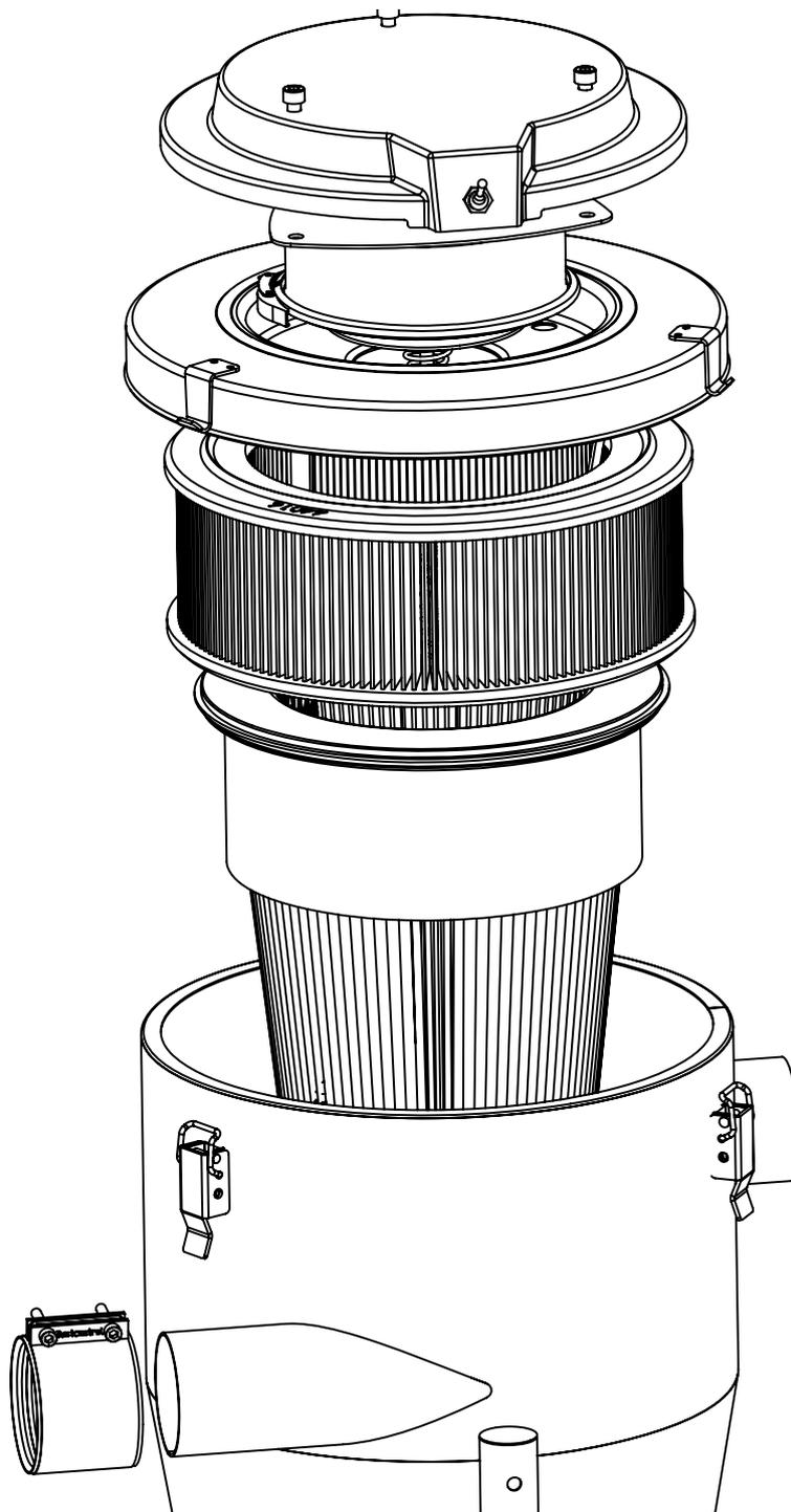
Fit the HEPA filter so that it is located centrally and check that the seal is evenly seated by rotating the filter.
